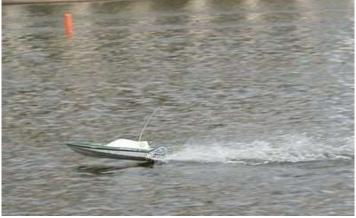
Limited Spec Mono Club SPEC: Plastic V mono, no steps or ride pads 19t Spec motor 6 cells - 7.2 volts max Common hulls: BBY Oval Master WH Force 21 and Force 22 Common Motor: Trinity Chameleon Common hardware: Fuller mono kit (1/8" shaft) Hughey hardware (1/8" shaft) Turn fin, motor mount, trim tabs Common props: Octura x431, x632, y531, y534
